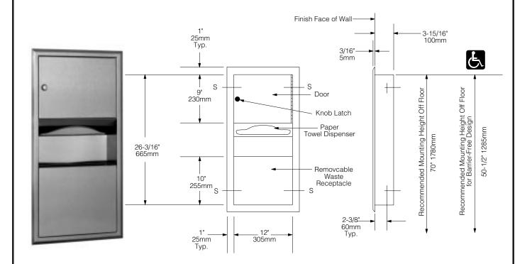
Rough Wall Opening 12-5/8" (320mm) wide 26-5/8" (675mm) high 4" (102mm) minimum recessed depth
